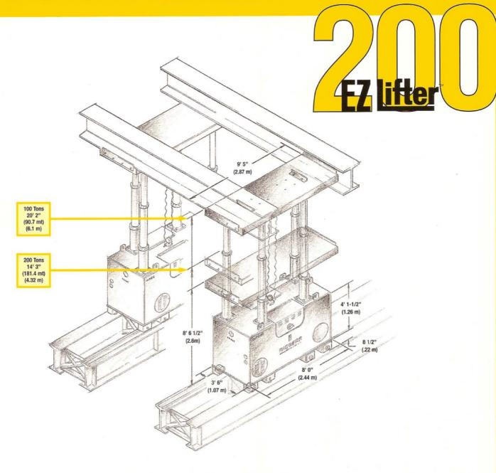
LIft Capacity 200 Tons @ 14'2" (4.3 m) Extension
