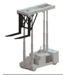
Turn the TriLifter into a 100 ton forklift with the addition of forks and a buttress.
