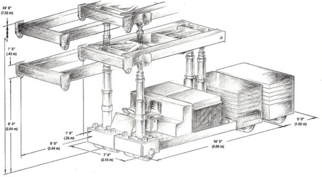
Maximum Lifting Capacity 65.0 Tons (58.97 Metric Tons)
